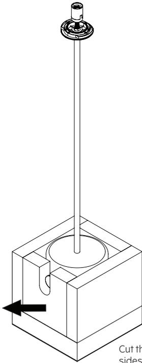
Cut the tape in the sides, and remove the part as shown.
